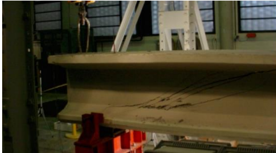
Figure 7: Case PB5. Details of the girder at failure. The picture is taken from (Choulli, 2005).
