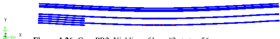
Figure 4-26: Case PB2. Yielding of bars #3 at step 56
