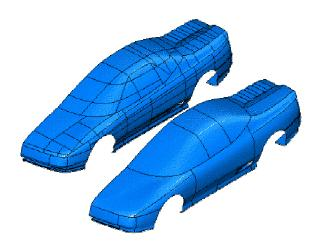
Using CADfix, poorly defined surface/face models can be transformed to clean solid models in minutes.
