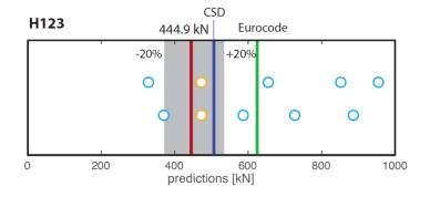
The results of the prediction of the Contest H123 girder showed a lot of variation in predicting the correct failure load, based on the NLFEA Guideline 2017, version 2.1. The reason of the different variations could be:
