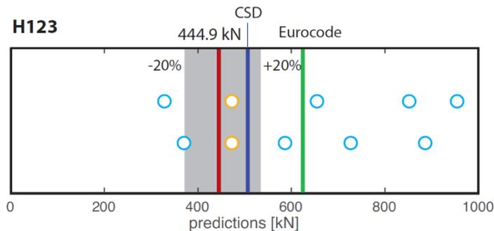
The results of the prediction of the Contest H123 girder showed a lot of variation in predicting the correct failure load, based on the NLFEA Guideline 2017, version 2.1. The reason of the different variations could be:
