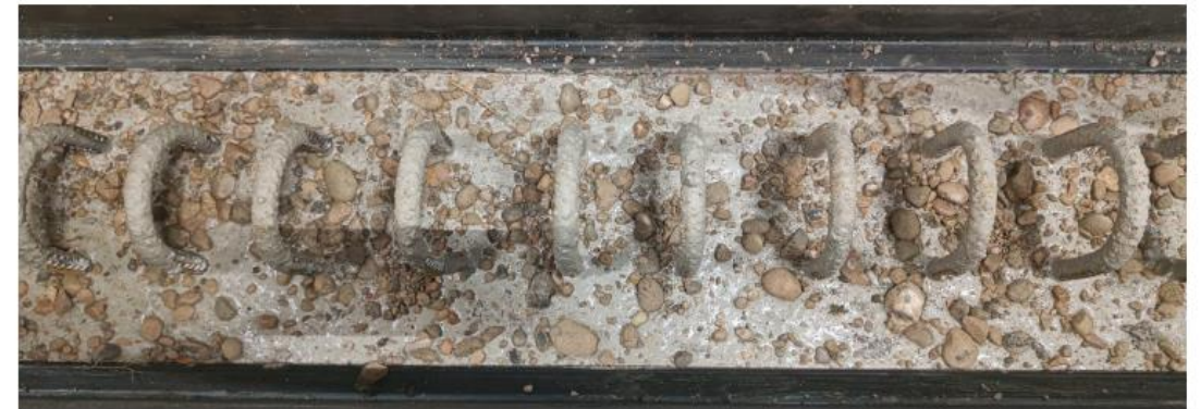
Figure 2: Interface treatment and hairpin reinforcement
