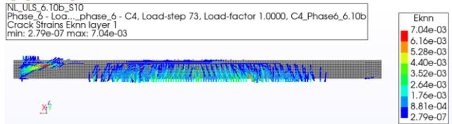
slight increase in development of shear deformation at 2.0xULS
