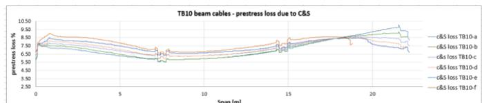
prestress loss due to C&S per cable along length
