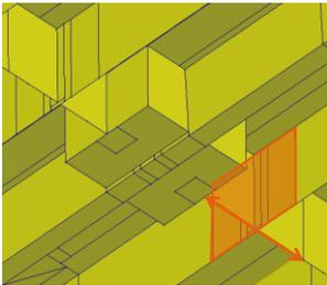
zone 'within' cross beam: width = c.t.c. girders = 1.4 m
