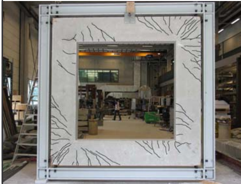
Experimental crack pattern
