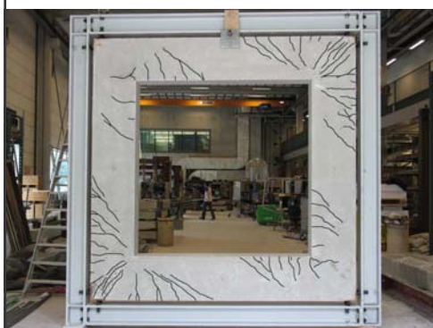
Experimental crack pattern
