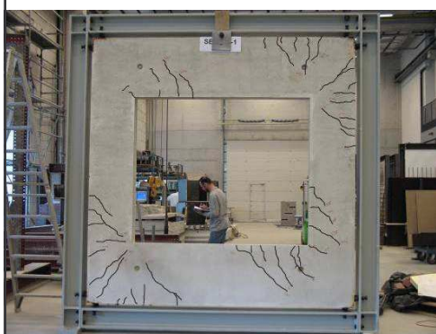
Experimental crack pattern
