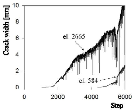
Development of crack width in elements 2665 and 584 in 'time'
