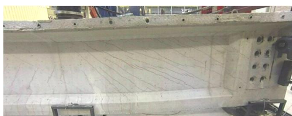
Girder #101 a/d = 2,7 Last step to failure
