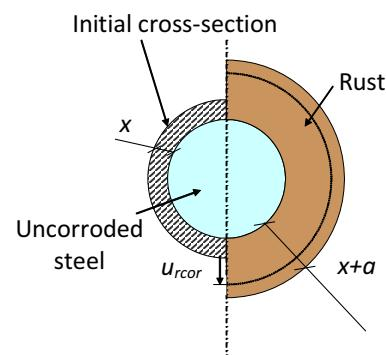
Strain in the rust depends on corrosion penetration  $x$ , expansion factor  $v_{rs}$ , and deformation  $u_{rcor}$
