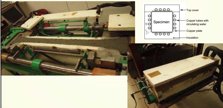
The situation in the structure's critical section can be tested with the right material, realistic temperature history and the right degree of restraint
