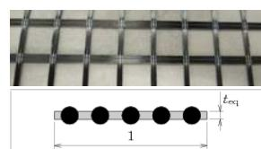
Figure 14.25: Equivalent thickness of reinforcement grid
