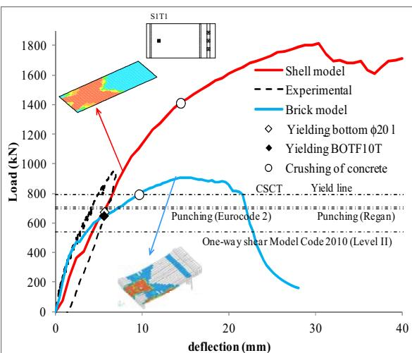
As expected the **shell model** is not able to properly describe the shear failure of the slab and substantially **overestimates** the capacity of the slab
