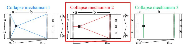
Yield pattern of collapse mechanism 2 in agreement with experimental crack pattern
