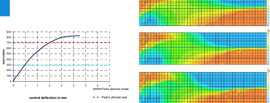
Figure 6.4:  $\sigma_{xx}$  over load steps 23 to 28, from 924 to 997 kN/m
