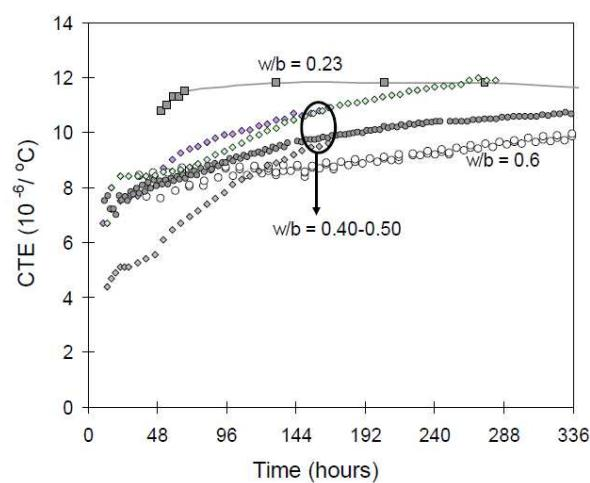
Fig. 17 Laboratory measurements of the coefficient of thermal expansion ( $\alpha_r = \text{CTE}$ ) over time for different concretes with variable water-to-binder (w/b) ratio. [19]
