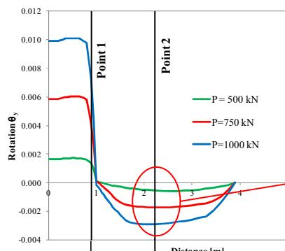
Rotation  $\theta$  = difference between the rotations of the slab at two points: **Point 1** and **Point 2**.
