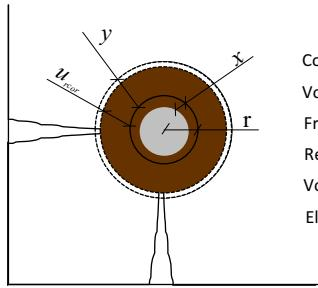
Corrosion penetration:  $x$
