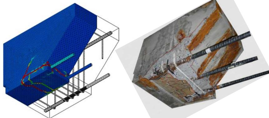
Corrosion products through cracks
