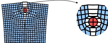
— Analysis, corrosion equal around the rebar
