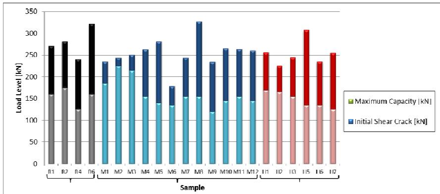
Initial shear cracking occurs in a lower level before the anchorage failure
