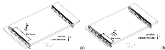
Fig. 17. Effective width  $b_{\text{eff}}$  determined from NLFE analyses for slabs S1T1 (a) and S4T1 (b).
